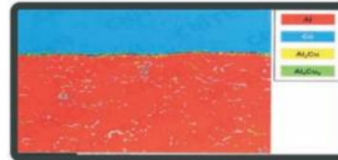
Interface Morphology of T2 Copper-1060 Aluminum Composite Plate
