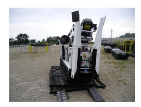
The EZ Hauler Xtreme with patent pending track extension system. This new track extension system allows the unit to retract to 35.5" and extend to an amazing 56". The new Xtreme EZ Hauler track system allows for unmatched stability when travelling on uneven terrain with your EZ Hauler, while still maintaining the ability to fit through a standard gate opening.
