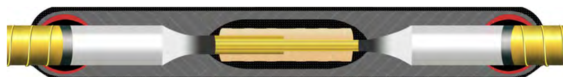
Using customized cable ferrule
